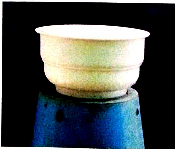
2. Container for leachate collection
